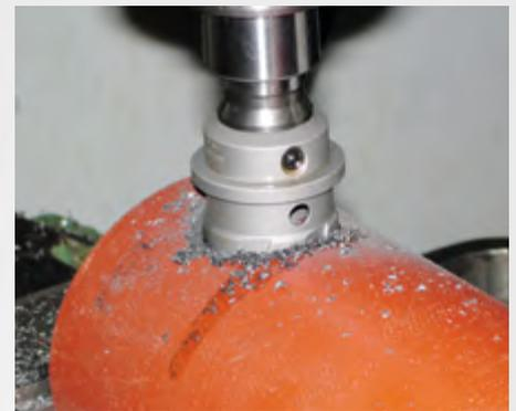
Bohren in Rohre
