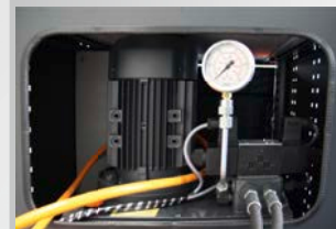
Dual-circuit hydraulic unit in cabinet base
