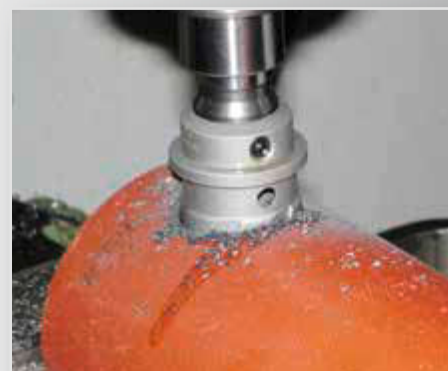
Bohren in Rohre
