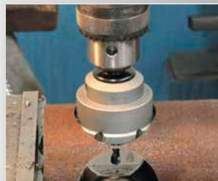
Bohren in Rohre
